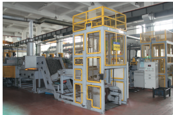
Continuous meshbelt furnace
