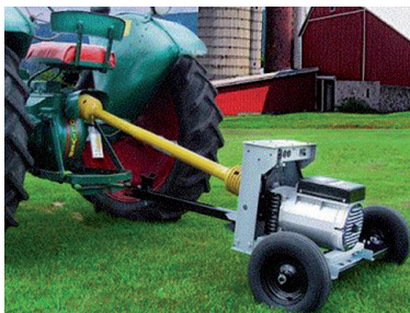
Tractor with an AC Generator
