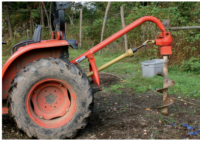
Tractor with a Post-hole digger
